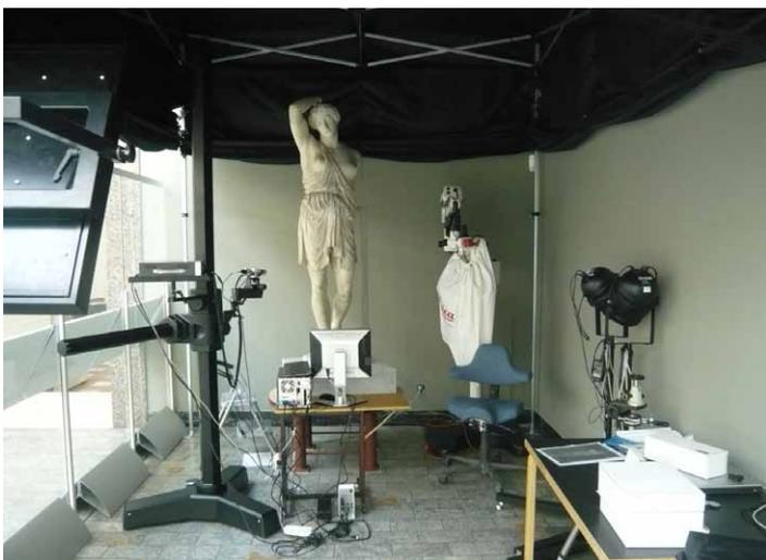
Fig. 3: The Sciarra Amazon mounted on the heavy duty turntable, with the Leica DVM5000 video microscope array and FOBA stand ready for action. In the left foreground a UV-lamp, right foreground LED-lamps for VIL-imaging. In the right background the Leica M651 operations microscope.
